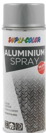
Aluminium coating with reliable adherence on metal, wood, glass, hard plastics etc. Protects from corrosion and weather influence. Protective coatings on exhaust systems, heat pipes in tiled stoves, heat-loaded stovepipes in workshops etc.. Heat-resistant up to 600°C. No color change when exposed to temperature. 99,5 % pure aluminium according to DIN EN 576:2003.
