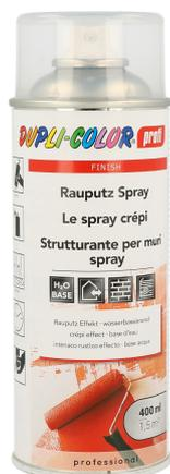
Creates an individual surface structure, similar to a rough plaster. It is an exclusive, water-based polyurethane dispersion, which is suitable to repair and adapt a textured plastering. It can be used on misc. surfaces, such as concrete, gypsum plasterboard, sheetrock, wood etc. Can be overcoated with all dispersion paints.
